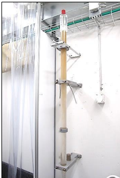
Figure 4-5. A typical settling pattern of soil particles through the water column: coarse particles settle fastest, while the fine particles stay suspension at upper part.
