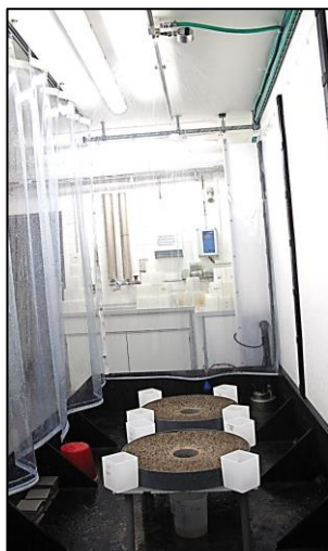
Figure 3-1 Conventionally farmed soil (CS) and organically farmed soil (OS) in round flumes were simultaneously subjected to simulated rainfall. The white boxes were used to monitor the rainfall intensity. This picture was also presented in (Hu et al., 2013a).
