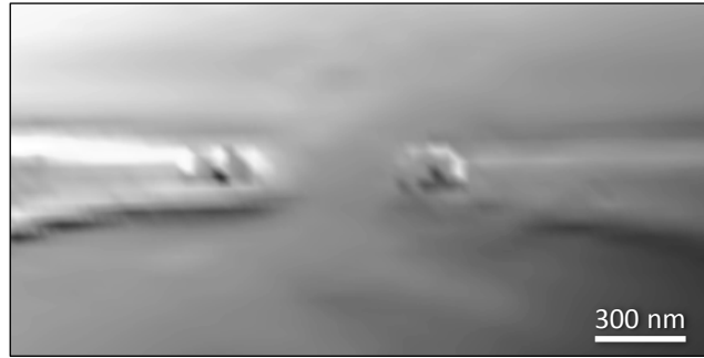
Figure 3.4 | Scanning probe micrograph of the QPC. The image shows the QPC split gates and is obtained by using the cantilever as a non-contact AFM probe, situated z = 80 nm above the sample surface. Data were processed with WSXM software [106].
