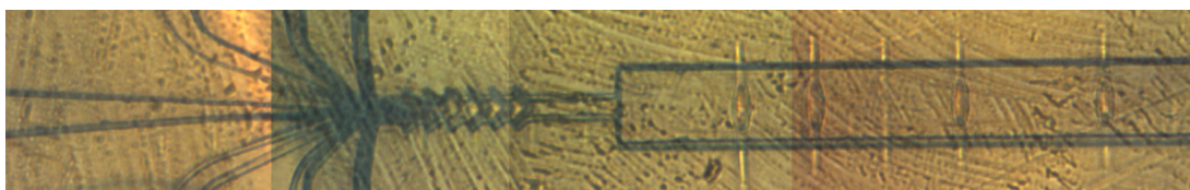
Figure 4.13: Photograph of the microfluidic mixing device after measurements at the synchrotron. Beam damage is clearly visible and resulted in changing background signals during preliminary measurements. As a consequence, the integration times have been drastically reduced in later experiments.
