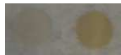
Figure 4.22: Sintered \text{TiO}_2 electrodes treated either with only CuI (on the left, \text{TiO}_2+\text{CuI} ) or with ALP1 and CuI (on the right, \text{TiO}_2+\text{ALP1}+\text{CuI} ). The colors of the cells are clearly differing.
