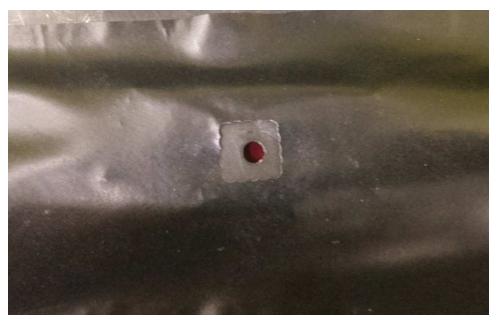
(b) DSC with mask taped off by a bigger piece of scotch tape.
