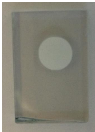
Picture 8-15: Photograph of an electrode consisting of 5 layers ZnO and one TiO 2 scattering layer.
