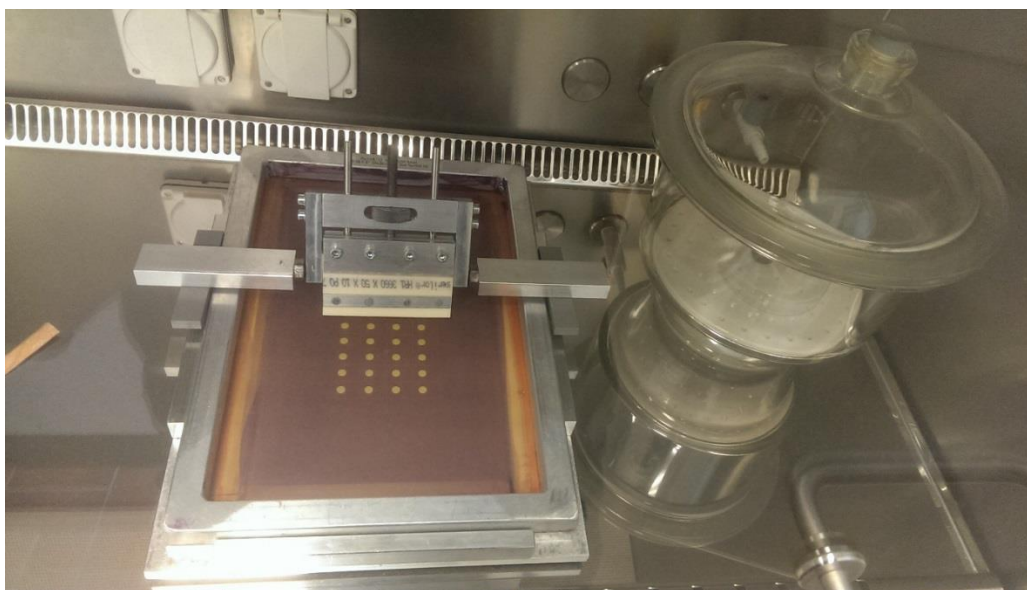
Picture 8-1: Screen printing device with mesh, squeegee and desiccator (for EtOH vapour treatment) inside a clean bench. Photo taken by Ewald Schönhofer.
