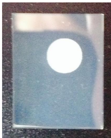
Picture 8-20: Photograph of an electrode consisting of 5 layers ZnO and one SiO 2 scattering layer ( SPP2 ).
