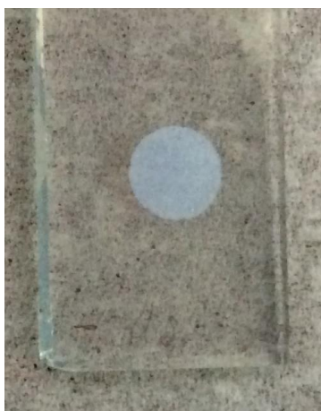
Picture 8-5: Sintered electrode consisting of five layers of ZnO.
