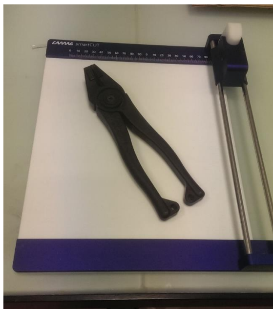
Picture 8-2: CAMAG smartCUT glass cutter and pincers. Photo taken by Ewald Schönhofer
