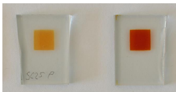
Picture 6-1: Image of electrodes incorporating [( 10 )Zn( 22 )]Cl 2 (left) and 24 (right). Picture taken by Danielle Hayoz.
