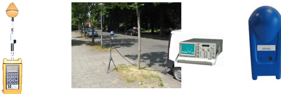
Figure 5: Different measurement devices for assessing RF-EMF exposure. Broadband probe (left), spectrum analyzer (middle) and exposimeter (right).
