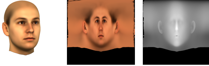
Figure 4.2: Projection of a 3D mesh to a 2D domain. On the left, the 3D mesh. The middle image is the projection of the texture, while the right image is a grey-coded representation of the range values. The range values are enough to recover the geometry, since the image coordinates provide the angle \phi and the height y . The black areas in both images are the void pixels.
