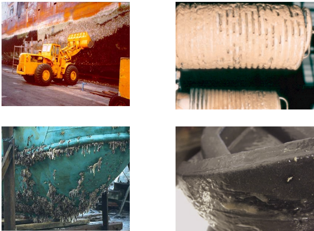
Figure 3.1: Left, heavily fouled ship hulls. 2 Upper right, heat exchangers of a pump after six month of operation. Lower right, biofilm formation on a valve in a drinking water system. 7
