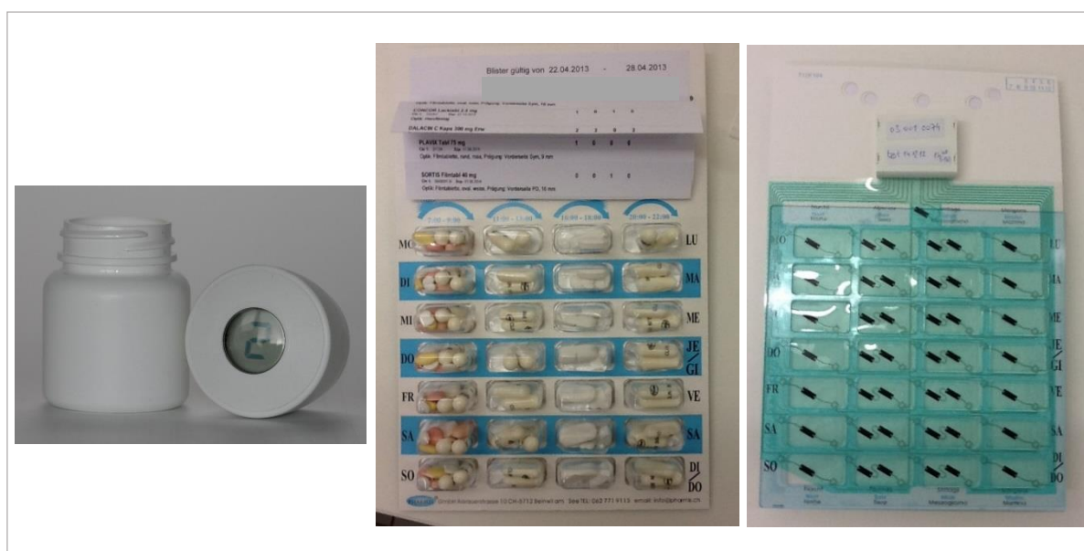
Figure 5. Medication Event Monitoring System (MEMS®, left) 73 ; multidrug punch card, front (middle); multidrug punch card, back with affixed POLypharmacy Electronic Monitoring System (POEMS, right).
