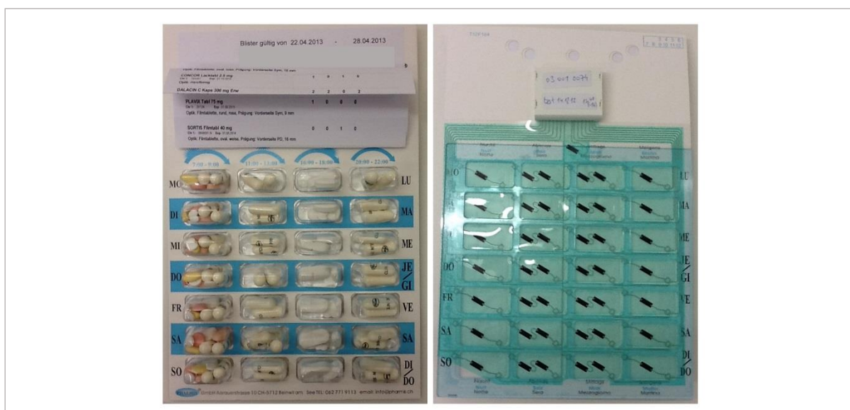
Figure 1: Electronic multidrug punch card front (left) and back with affixed POLYpharmacy Electronic Monitoring System (POEMS; right).
