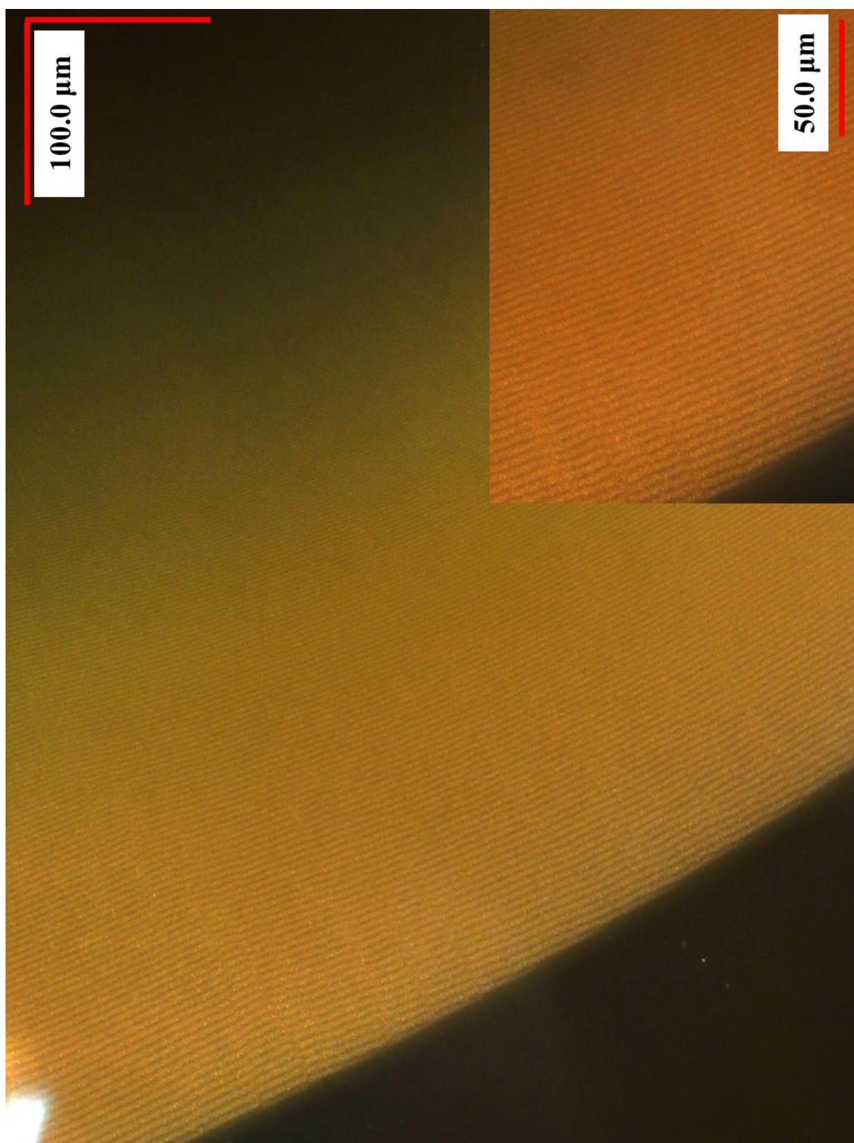
Appendix B, Image 4: Highly periodic precipitation bands found in samples prepared with sodium hydroxide (0.1 M NaOH) as base. Overview image (100 μm scale bar) and zoomed in image at the end of the precipitation zone (bottom right), with a 50 μm scale bar.
