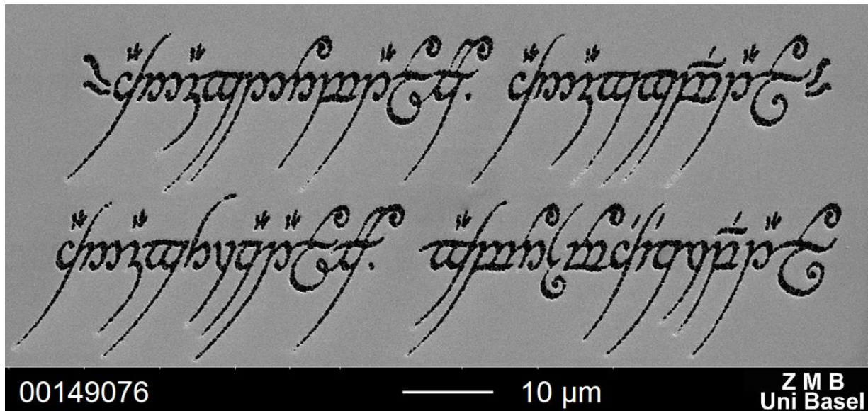
Picture 1: SEM-FIB nanolithography used to write J.R.R. Tolkiens: One Ring to rule them all, ... , in elvish tengwar letters on a gold surface. Text was taken from “The Lord of the Rings” .
