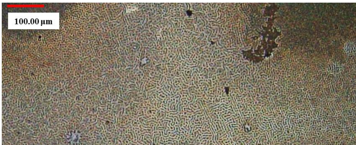
Image 5.10: Optical image of a sample also sintered at 360°C for 12 h, where rearrangement was observed.
