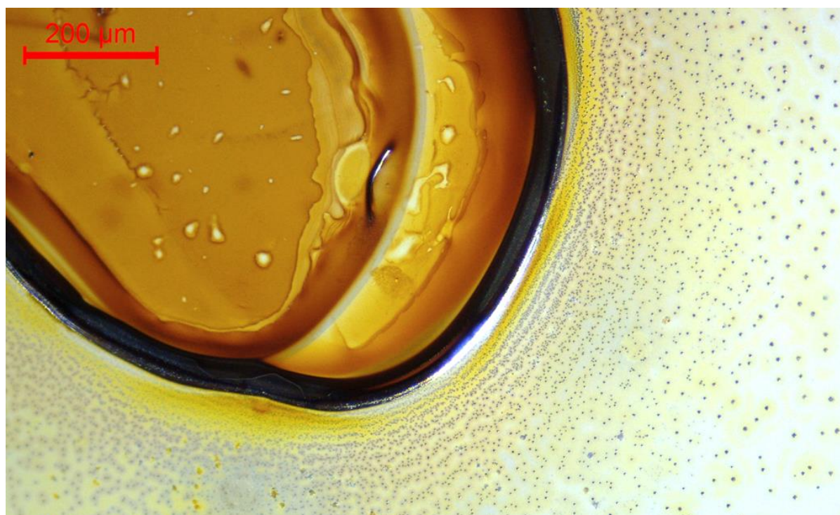
Image 6.8: Optical image of the precipitation bands observed in the \text{AgNO}_3 / \text{Na}_2\text{WO}_4 WETs system.
