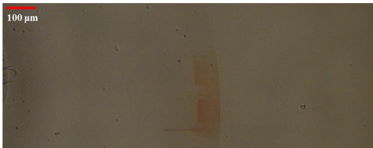
Image 4.1: Optical image after laser profiling: Middle left: stamp interaction site, middle brown: end of precipitation zone and place where the laser irradiated the sample.
