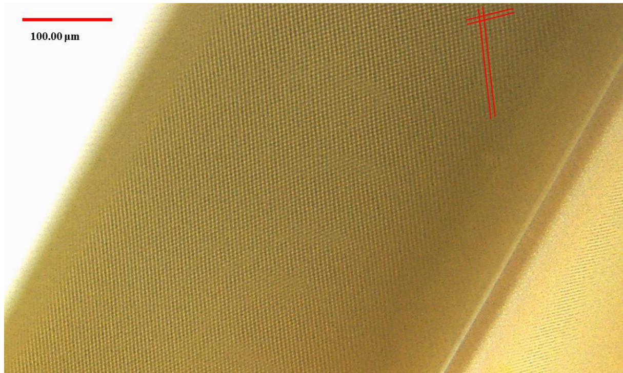
Image 5.13: Optical image of a meso scale grid prepared by using the new fine structured silver Liesegang precipitation system.
