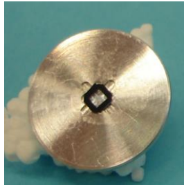
Image 2.5: Special vacuum chuck for \text{Si}_3\text{N}_4 membranes, which applies the vacuum only on the Si-frame edges (black).
