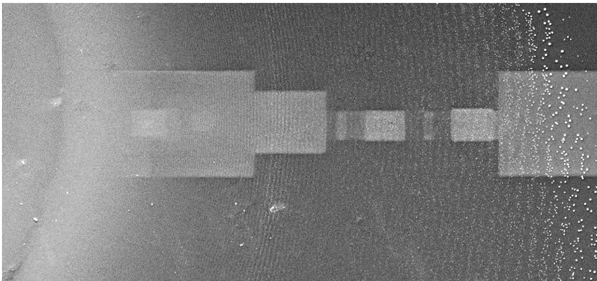
Image 5.2: SEM image showing where SEM measurements were performed (bright quarters). Left part: close to the stamping core, right part: close to the precipitation propagation front.
