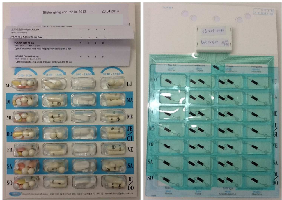
Electronic multidrug punch card front (left) and back with affixed POLymedication Electronic Monitoring System (POEMS; right).
