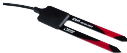
Figure 2.4. Decagon's 10HS soil moisture sensor
