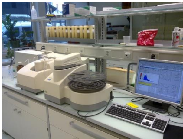
Figure 2.9. Measurement of soil and sediment particle-size using the Malvern Mastersizer 2000 analyzer
