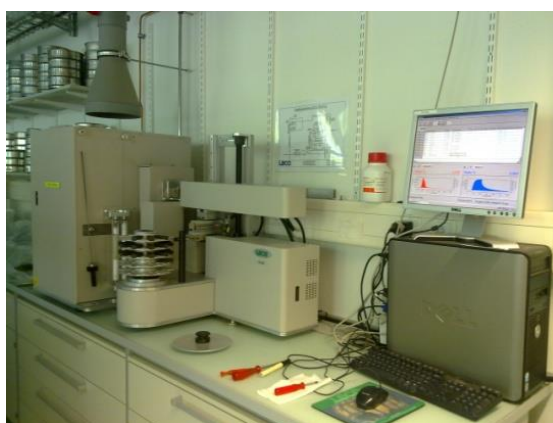
Figure 2.10. Measurement of TOC and CaCO 3 using LECO-RC 612
