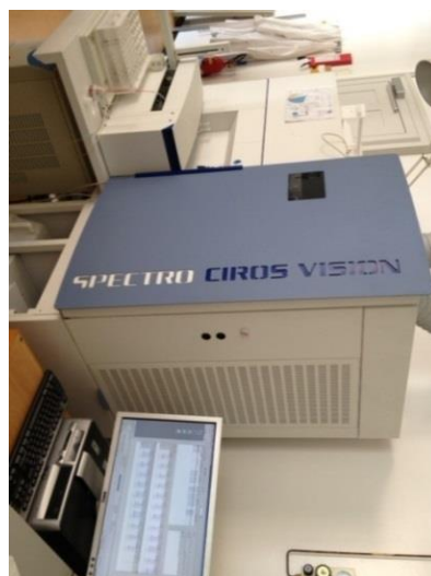
Figure 2.12. Measurement of P and K using ICP Spectro Ciros Vision
