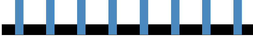
Figure 9.1: The figure shows a quantum wire (black) of length L with negatively charged gates (blue) forming a superlattice potential. Due to the induced charge density modulation a bound state at each wire end can emerge.
