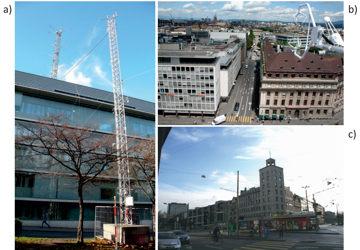
Figure 3.3: Photographs of the measurement sites: (a) Basel Klingelbergstrasse, showing the street canyon tower and the rooftop tower; Basel Aeschenplatz showing (b) the EC system and the view over the city approximately to the north and (c) the view across the Aeschenplatz toward the Turmhaus building with the instrumented flagpole on top.
