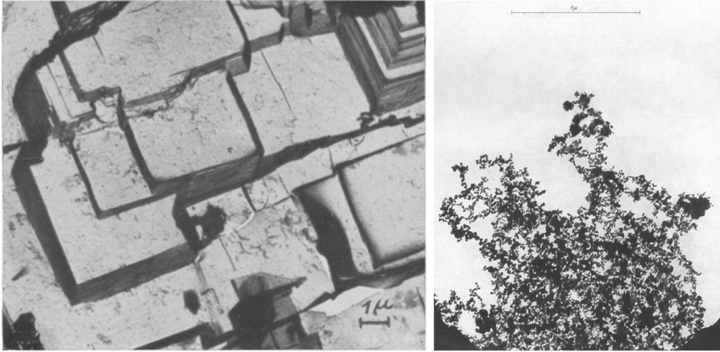
FIGURE 1.4: By the time of world war II, electron microscopy was already a developed technique as shown in on some example images. Left: Electrolytically generated oxide imprint of etched aluminium in TEM [20]. Right: Iron oxide particles from iron-pentacarbonyl in SEM [21].
