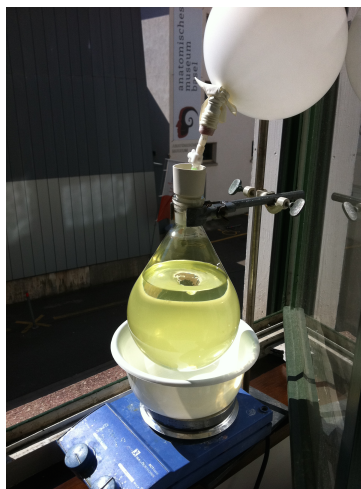
Figure 2.4: Sunlight experimental set-up of the Wolff rearrangement.
