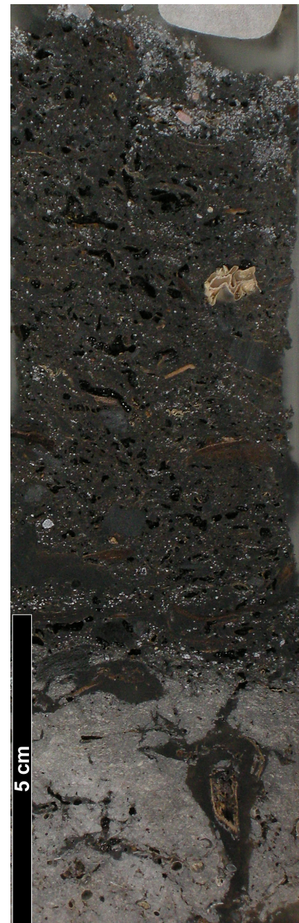
Fig. 6 The polished section of the profile column LALU 2; at the bottom the grey lake marl is overlain by the dark cultural layers composed mainly of organic matter. The upper part consists of grey sand
