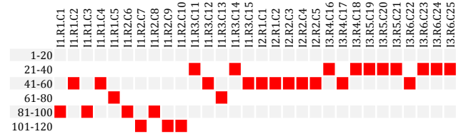
Figure 7. Fourth use case: Node failures over an 8-month period from 01-09-2014 to 30-04-2015. Chassis in the same rack and racks in the same island exhibit spatial correlation even over a longer period of time (no temporal correlation is made here).
