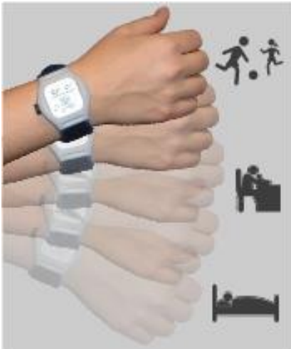
Figure 1.2. Wrist-accelerometry In the EPHECT I-Study, an accelerometer from SOMNOwatch™, Randersacker, Germany) was applied to measure PA and sleep objectively.
