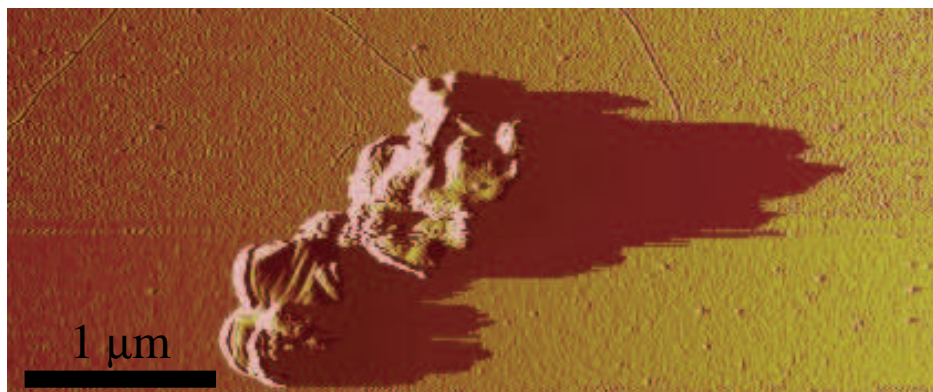
Figure 2.13: Catalyst clusters disturb AFM measurements (obstacles cause shadowing).
