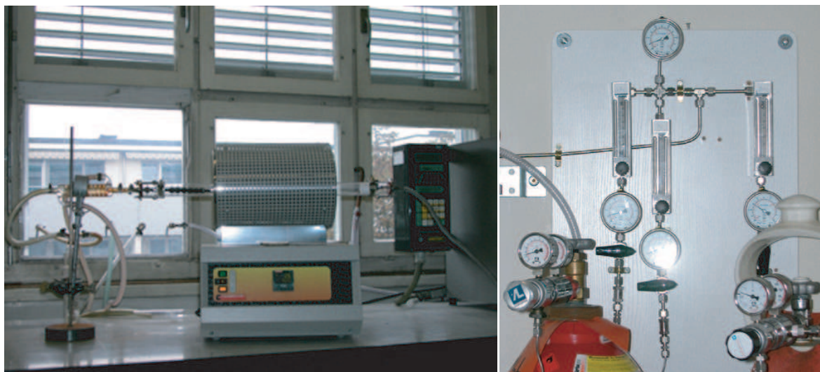
Figure 3.1: The CVD oven and the actually used gas system.
