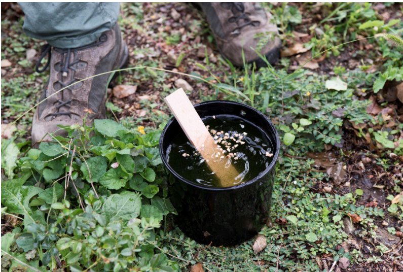
Figure 1.4: Ovitrap in Ticino, Switzerland. Mosquitoes are attracted by the water in the container and deposit their eggs on the wooden slat. The Bti granules in the water are lethal to mosquito larvae and prevent adult emergence.
