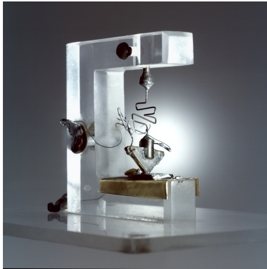
Figure 1.1: An enlarged replica of the first Germanium point-contact transistor (Figure taken from Ref. [25]) consisting of a triangle with gold contacts, that is pressed upon the n -type germanium. Below a copper contact serves as base terminal.
