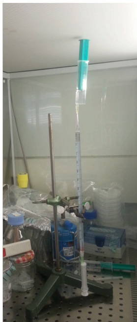
Figure 29. Digital image of the column set-up used for nanomimic purification to avoid high endotoxin contamination. Sterile 10 mL plastic pipettes, syringes, needles, and freshly cleaned column material (washed in 0.5 M NaOH overnight) had to be used to yield nanomimic samples with endotoxin contamination below 0.005 EU/mL.
