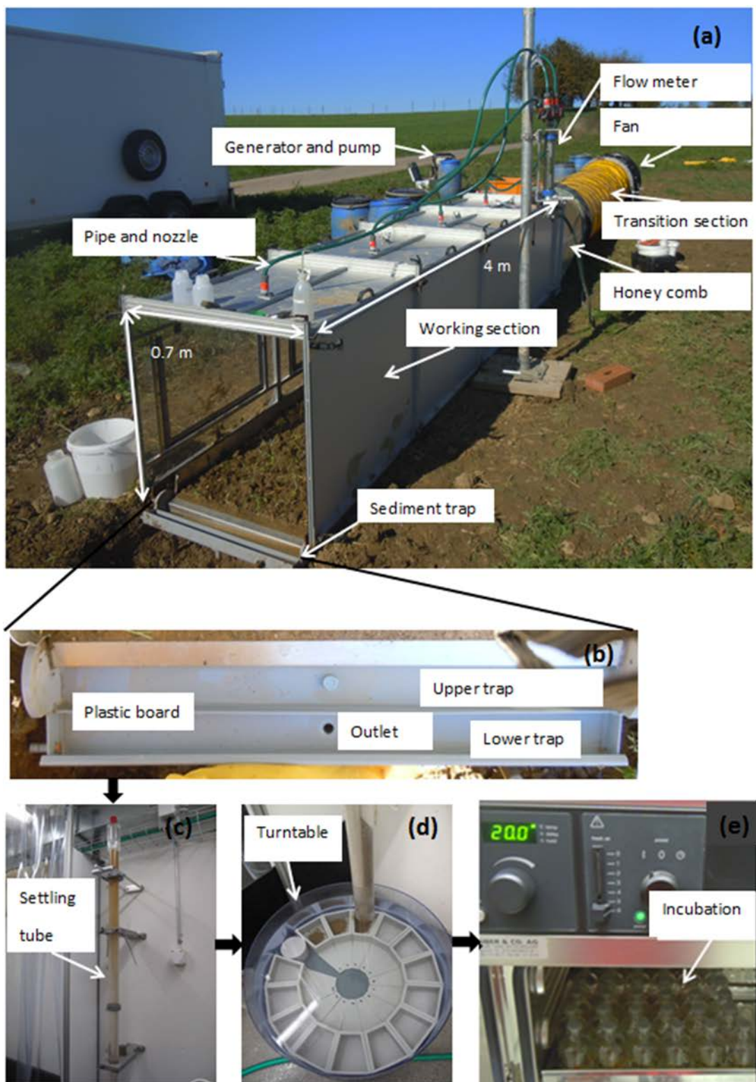
Figure 2.1 The experimental procedures: the rainfall simulation with a portable wind and rainfall simulator (PWRS) (a), the sediment trap (b), the settling tube apparatus (c), the turntable to collect the fractionated sediment (d), and incubation of the fractionated sediments (e).
