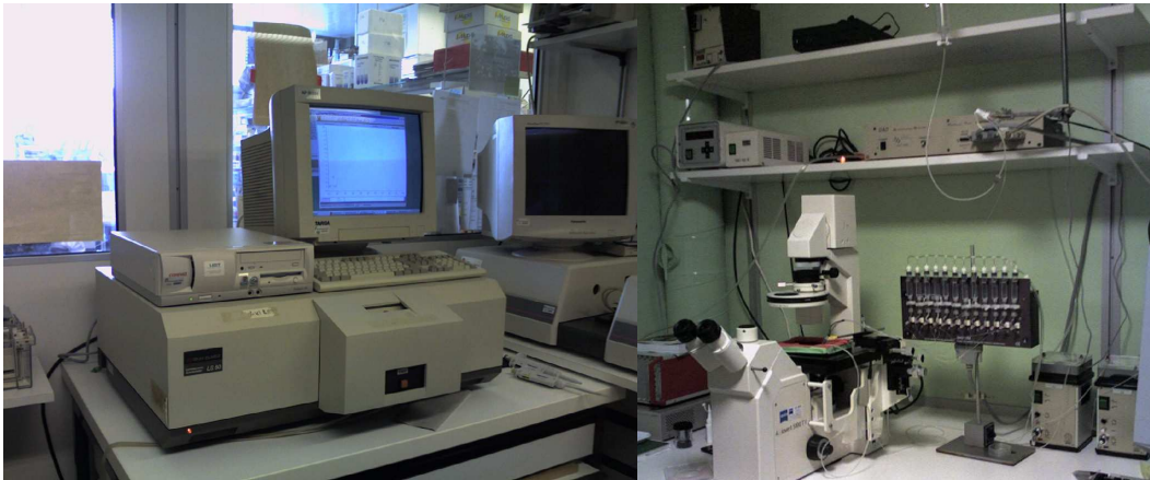
Figure 2-1: Systems used for \text{Ca}^{2+} measurements: in population of cells with a Perkin Elmer LS-50 spectrofluorimeter (left) and at single cell level by inverted microscopy (right).
