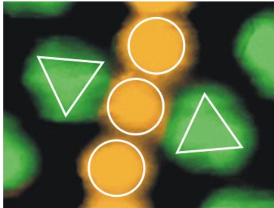
Figure 3.5.: Self-intermixed monolayer on Ag(111) and its molecular components. Artificially colored Scanning Tunneling Microscopy image of the basic unit of the molecular stripe pattern with superimposed schematic contours (SubPc green, C_{60} yellow). Individual components can be identified by size and shape. Scan range 4.3 nm x 3.2 nm. V_{bias} = 1.3 V, I_t = 20 pA.
