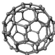
Figure 3.4.: Structure of C_{60} . The diameter of the carbon cage is approximately 7 Å.
