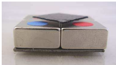
FIGURE 2.1 | Pyrolytic graphite levitating above permanent magnets due to the repulsion of magnetic field by the graphite.
