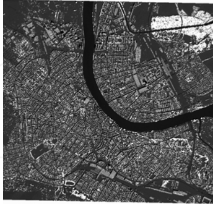
Figure 10. DART reflectance image for an NIR band (864.6 nm), over the city of Basel, corresponding to a Landsat-8 image, with erroneous (but realistic) optical properties used as input.
