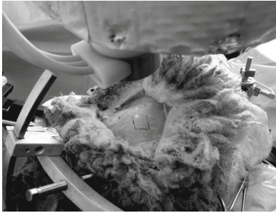
Fig. 8. The laser system performing a navigated cut on a sheep head.
