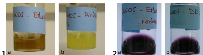
Pic. 4.18.5: Aspect of the vesicle preparations with the AU method 2 on the moment of preparation, 1a) standard method, 1b) direct dispersion method and after preparation, a) standard method, b) direct dispersion method..
