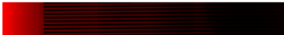
Figure 4. Low concentrations of proteins in solutions tend to deplete by surface adsorption with increasing distance from the filling port. The length of the depletion gradients can be used to calculate the adsorption time of proteins. [fig. from ref. 69]
