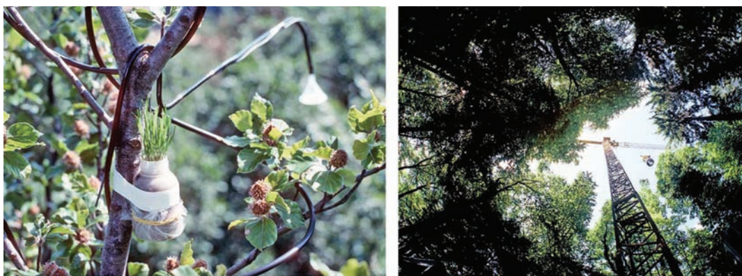
Fig. 1. Canopy CO 2 release by a web of porous tubes (left), with “iso-meters” (front) and gas sampling lines (back) for control, all operated from a 45-m-high crane (right).
