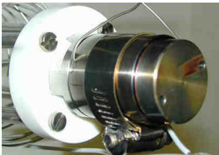
Figure 2-3 Photograph of the oven (outer shield and ionizer have been removed).
