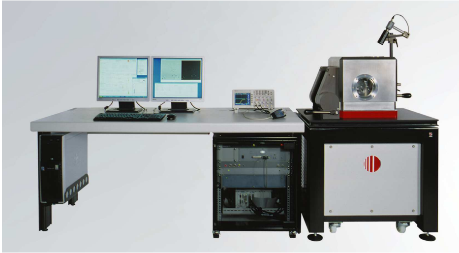
Fig. 2.10: Overview of the hr-MFM instrument including from left to right: The Acquisition computer running the software Scan Director , the electronic rack including the NI Real Time System TM , an oscilloscope, and the high vacuum chamber including the microscope itself 76 .
