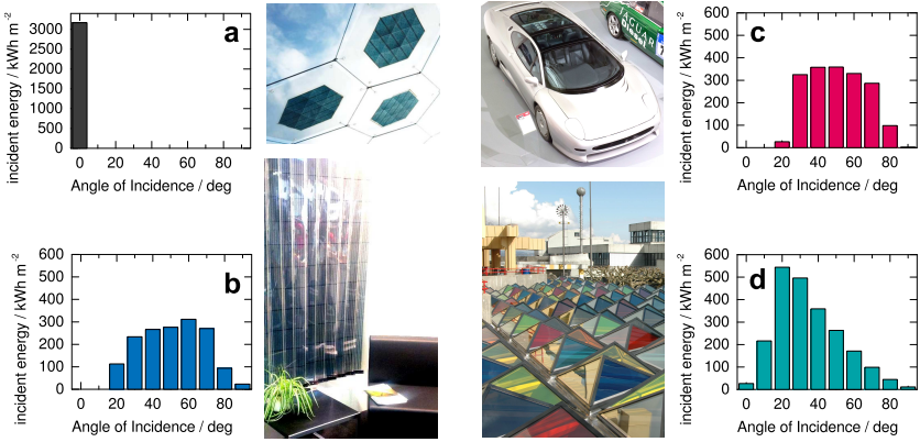
Figure 7.3: Various application planes and their irradiation. a Shadings, which are always pointed towards the sun (picture taken from Ref. [54]) b South-oriented facade or window blind (demonstrator of the SUNFLOWER project at LOPE-C conference, 2016) c Horizontal ceiling of buildings or cars (picture by Morio 4 ) d South-oriented building-elements, installed with a tilted angle. (Famous foyer glas ceiling by Otto Piene at the University of Konstanz)
