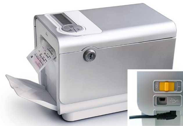
Figure 27: Remote-controlled, electronic dispenser, Medido®, used in this study as specific electronic medication management aid for the unit-of-dose pouches. Notes: Height \times width \times length: 140 mm \times 140 mm \times 225 mm. Weight: 1,486 g. The inset shows the power cord.
