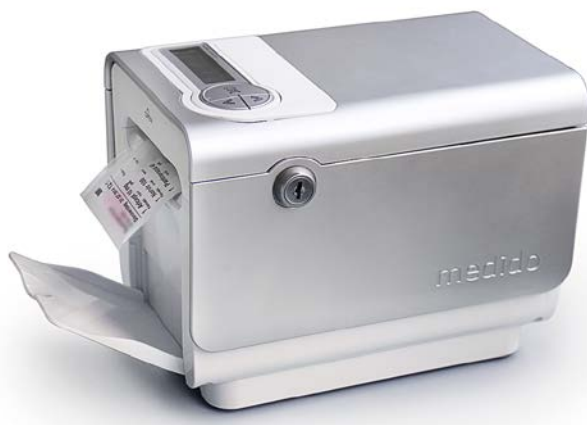
Figure 10: Remote-controlled, electronic dispenser for the unit-of-dose pouches Medido® used in this study as specific e-MMA with power cord in lower right corner (height x width x length: 140 mm x 140 mm x 225 mm, weight: 1486 g)
