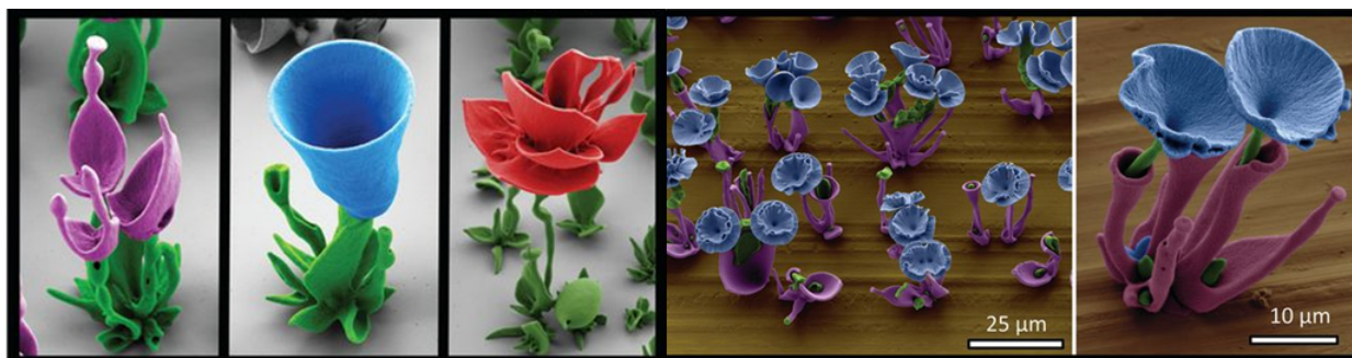
Figure 7. Stack of different morphologies on top of each other. The scanning electron micrographs are false-colored to mark parts of the structure grown in different steps. \text{SrCO}_3\text{-SiO}_2 vases (purple) containing \text{SrCO}_3\text{-SiO}_2 stems (green) that were subsequently opened with a \text{CO}_2 pulse (blue). [Adapted with permission from ref. 27. Copyright 2013. American Association of the Advancement of Science.]
