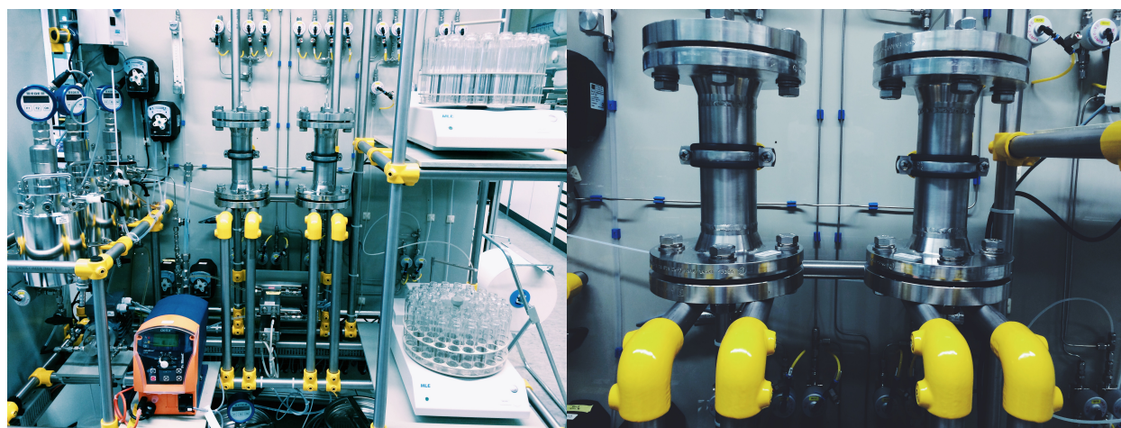
Figure 48. Pilot plant for the recovery of phenolic compounds, (left: overview of the pilot plant; right: two reactors containing the CDP).
