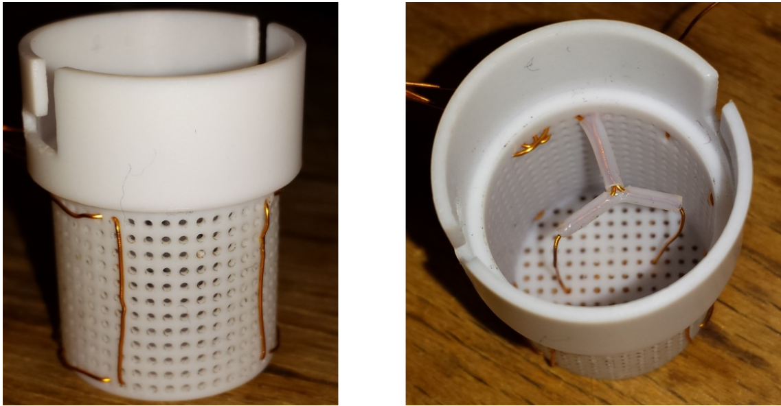
Figure 2.22.: NMR coils as of May 2015. Left-hand side: surface coil, right-hand side: in-beam coil. Figure taken from [77].
