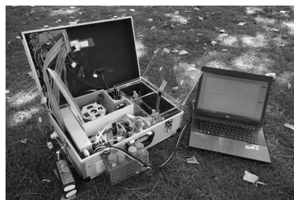
Figure 2. Photograph of the instrument. The syringe pump and valves are in the front, the thermostatted compartment in the center and the high voltage compartments are to the right. All compartments have been opened.
