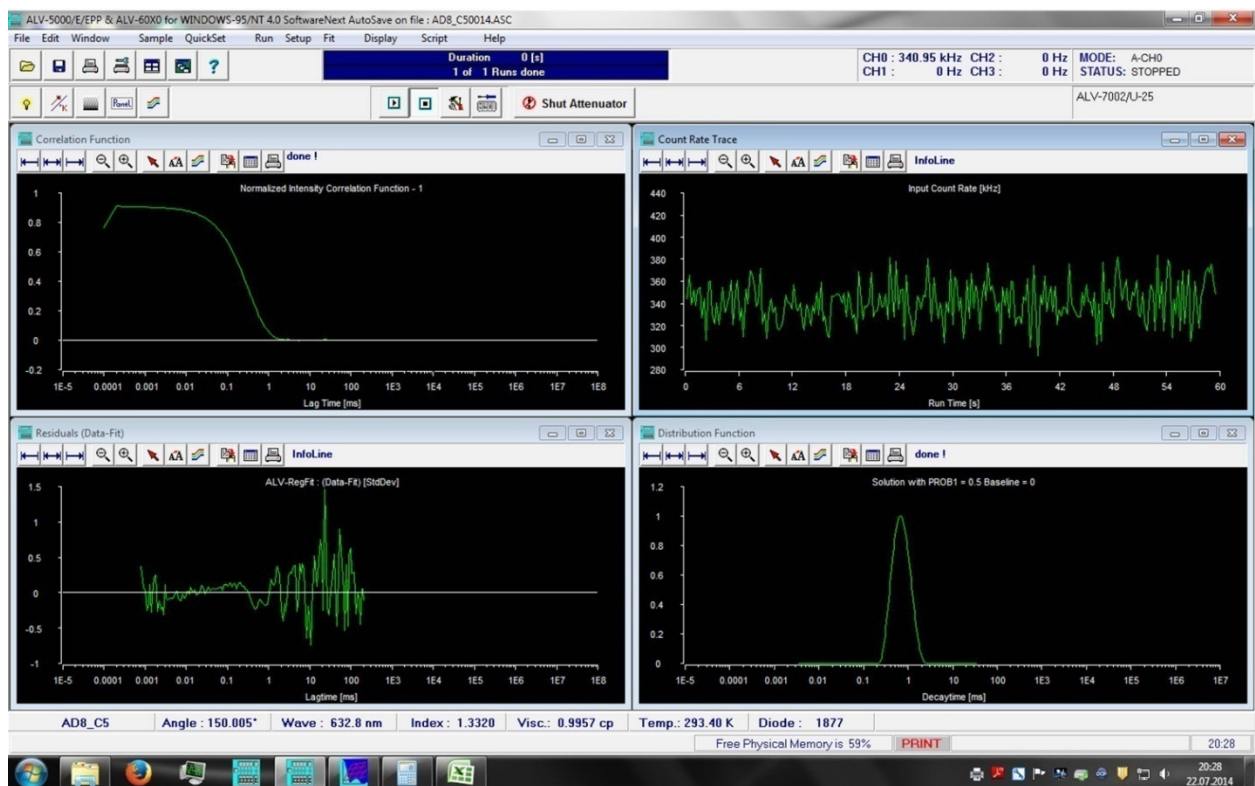
Fig. 53. Light scattering raw data for A 6 B 44 A 6 polymersomes with encapsulated pyranine, at a polymer concentration of 0.07 mg/mL: normalized intensity correlation function, count rate, plot of residuals from the data fit, and the distribution function.
