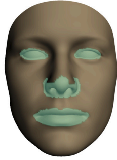
Figure 5.2: The green area depicts the non-hair mask prior. The mask is rendered to the image using the actual model state. The generated mask is used to lower the influence of frequently false positive hair predictions in the facial feature regions.
