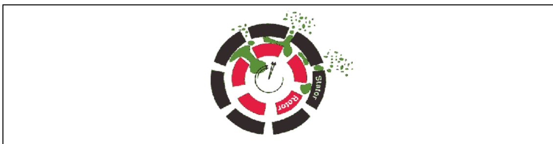
Figure 4 Cross-section of a rotor-stator aggregate
