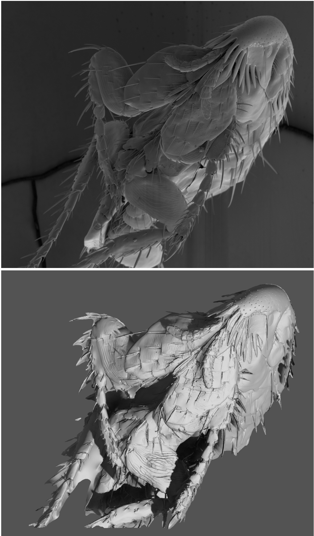
Figure 9.4: Left: SE image taken from the zero-tilt reference view. Right: Reconstructed depth map. The background was segmented using the result from chapter 8. Note the greatly improved shape of the head compared to the renderings in Figs. 8.4 and 8.5 on pages 99 and 100.
