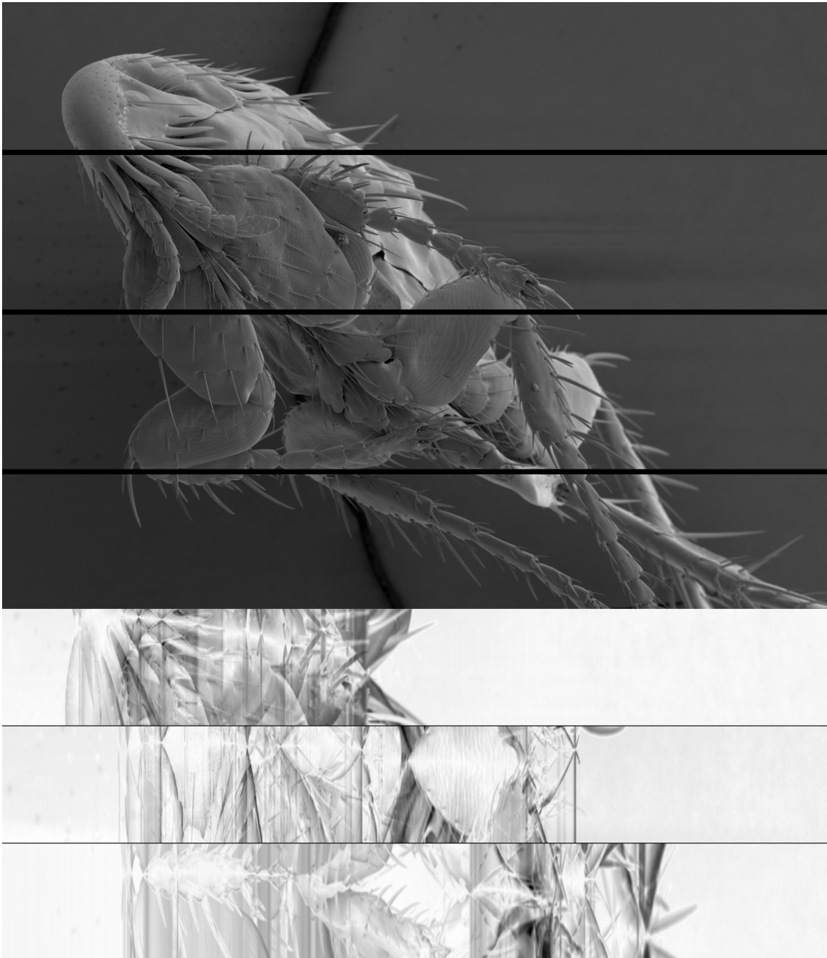
Figure 6.3: Slices through the filtered cost \bar{C}_z(x, y) at the y values indicated by the black lines, corresponding to the energy plots in Fig. 4.3 on page 40. Note the dramatic loss of quality in the wide-baseline scenario. Since only three images are used for the computation, the structure of those images is still visible in the cost slices.
