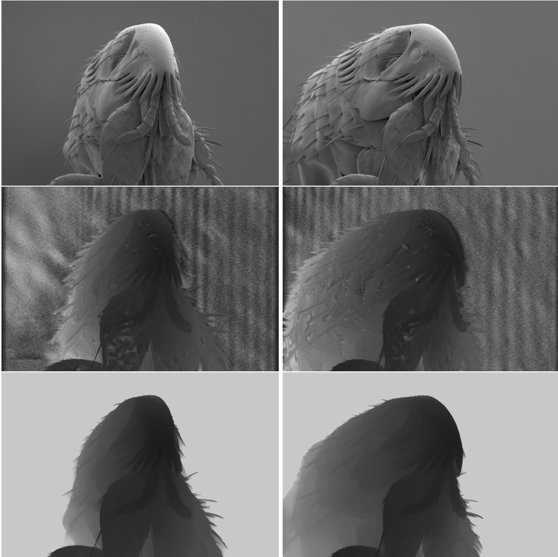
Figure 5.1: Depth map interpolation. Top row: the reference views; center: sparse depth maps; bottom: interpolated depth maps. Note that the noise in the uncertain areas disappears while the depth values near the edges remain constant.
