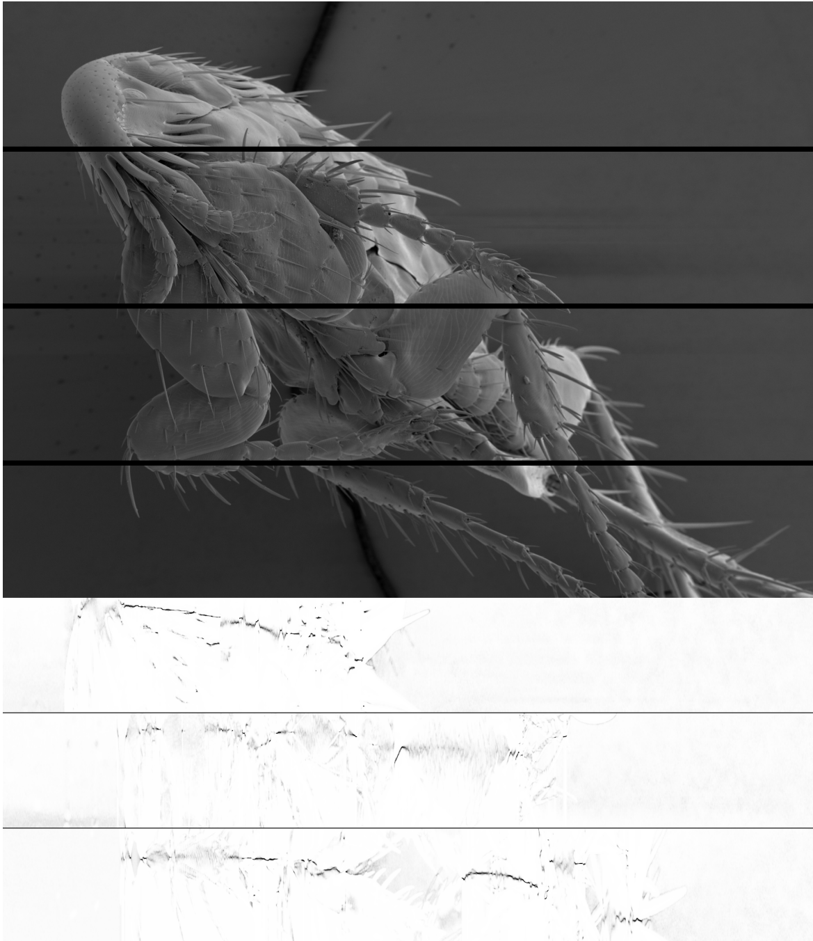
Figure 6.4: Slices through the probabilities p_z(x, y) corresponding to the costs in Fig. 6.3. Note the lower coverage and the increased number of spurious matches compared to the narrow-baseline scenario in Fig. 4.4 on page 41.
