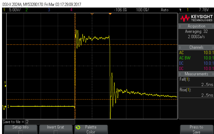
Figure 2.17: Measurement of rise and fall times: 2.5 ns each from 10% to 90%; amplitude is 25 A.
