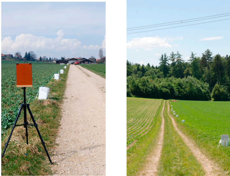
Figure 8. Measurement setup with the (white) measurement boxes in Iffwil ( left ) and Wiler ( right ). Only the right image shows the entire length of the measurement path with all nine boxes. Also shown in the left picture is the target table that was used with the laser distance meter to position the boxes and to measure the height to the conductors.
