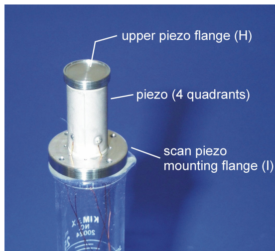
Figure B.3: Piezo with upper flange, bottom mounting flange and attached wires.
