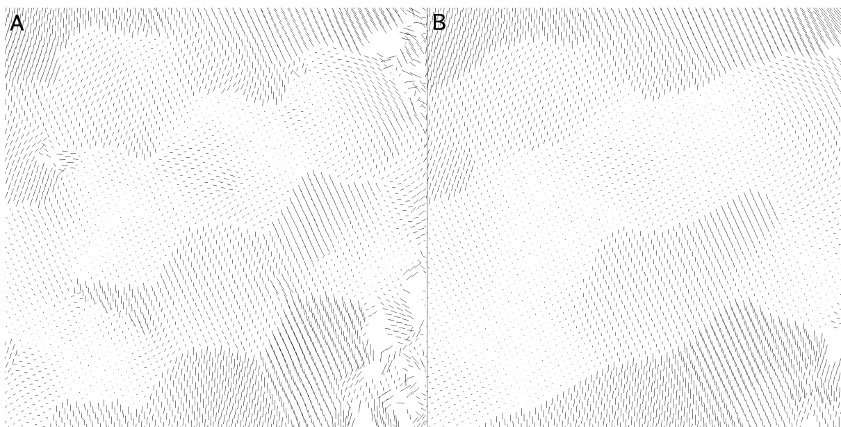
Figure 3.4: Displacement vectors during unbending with and without spot scan option. (A) Unbending with spot scan option deactivated (B) Unbending with spot scan option activated
