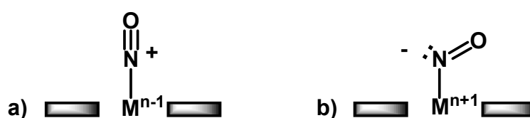
Figure 26: Illustration of the possible character of metal porphyrin-NO complexes. a) nitrosyl cation b) nitroxyl anion case.
