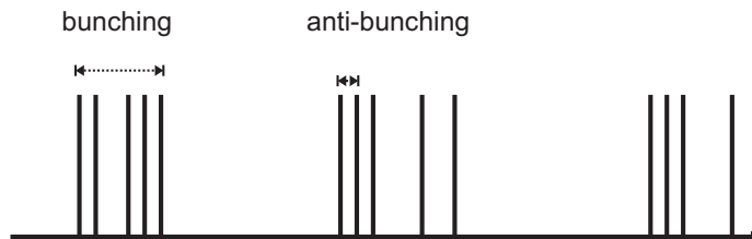
Figure 2.7: Single fluorescent molecules emit photons only after they have been excited, which causes anti-bunching of the emitted photons. By crossing over into the triplet state, the molecule exhibits some dark periods without emitting photons. This effect causes some kind of 'binning' of the photons, which is called bunching.
