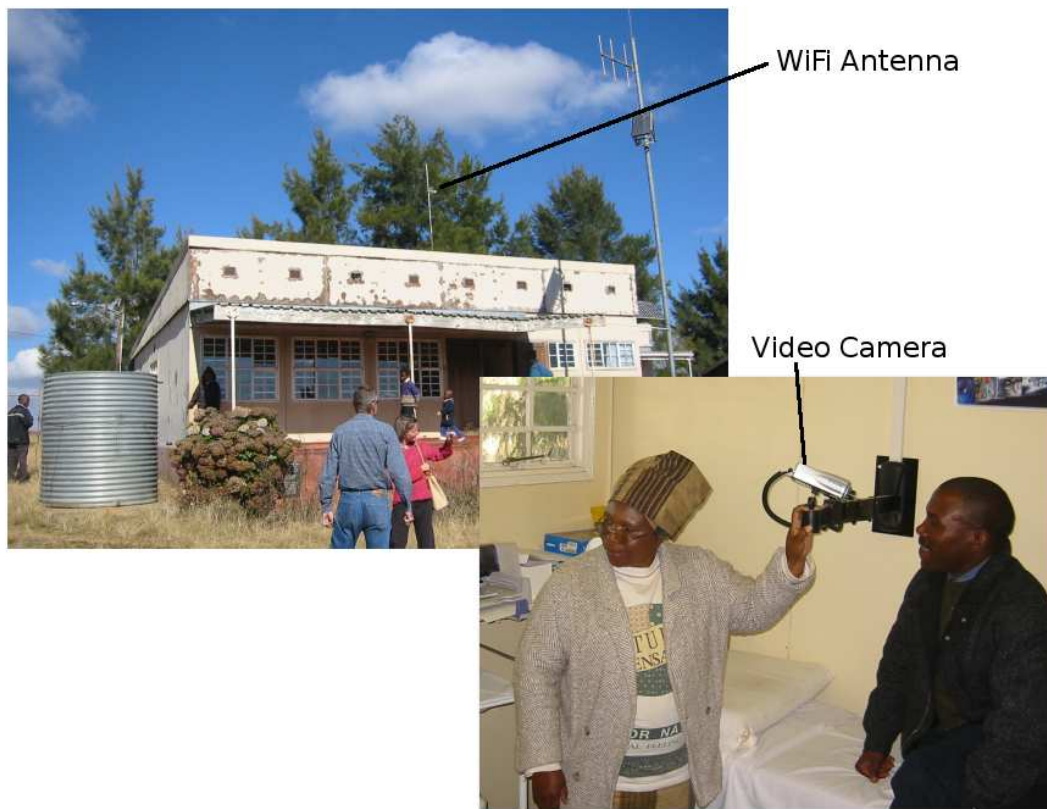
Figure 12.1.: The community clinic in Tsilitwa. Images captured with the video camera can be transmitted live over the wireless IP network (WiFi) to the Sulenkama Hospital, approximately 30km away.
